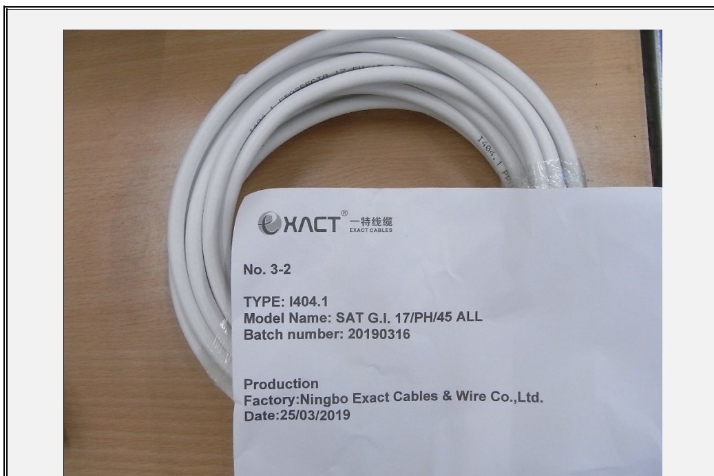
Foto No 2 : Cavo SAT G.I. 17/PH/45 ALL 1/1,13 mm BC stampigliatura : I404.1 PROSPECTA 17/PH/45 A SAT GAS INJECTED CEI-UNEL 36762 C-4 (U0=400V) Eca V712300179 + METRICA
